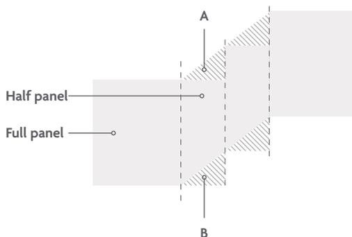
5. Place the template on the Lincrusta dado half panel and cut across the half panel. Put the cut-off triangle to one side – you'll need it later. **See Fig 06, Point B.**
